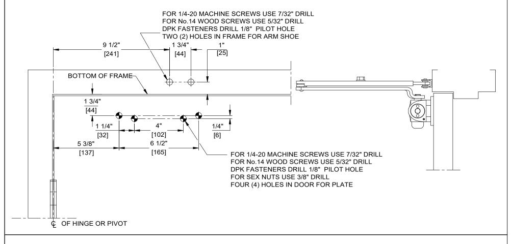
DOOR CLOSER MODELS: 8616 AF OR AR (NHO) REGULAR INSTALLATION (PULL SIDE MOUNT) WITH PLATES BP86, BP86FC
